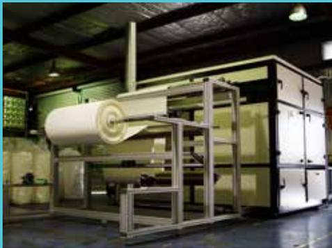
**Above** Revolution Fibres' state-of-the-art Komodo machine produces world-leading nanofibre products.
